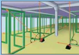
Aligning partition walls
